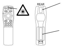
AVOID EXPOSURE-LASER RADIATION IS EMITTED FROM THIS APERTURE
